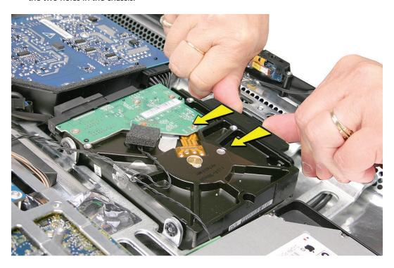
3. Connect the hard drive data and power cables to the hard drive.
